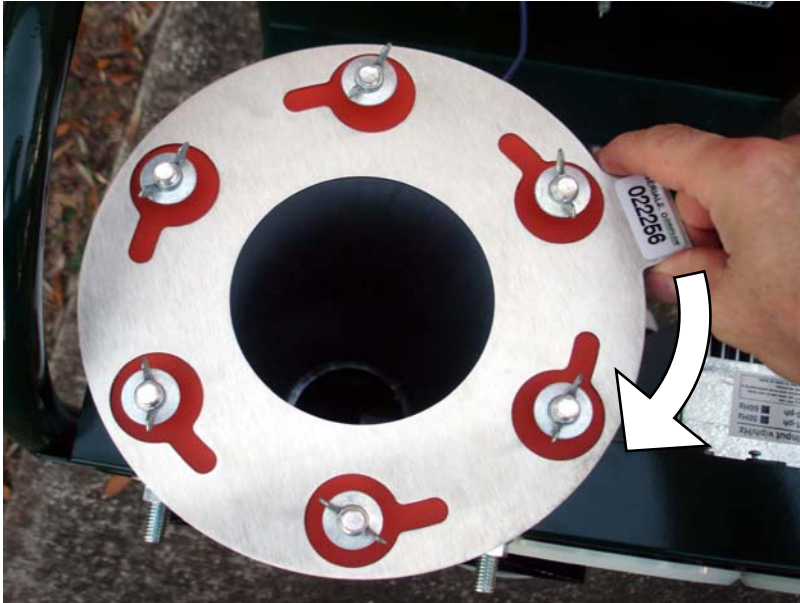
Figure 1 – Install Orifice Plate and then Rotate Clockwise
