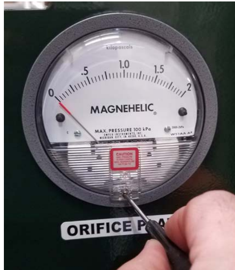
Figure 11 – Zeroing Analog Gauges
