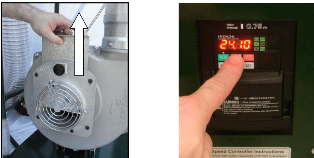
Figure 13 – Obtaining System Test Pressure (inlet slide model on left, VFD speed control model on right)
