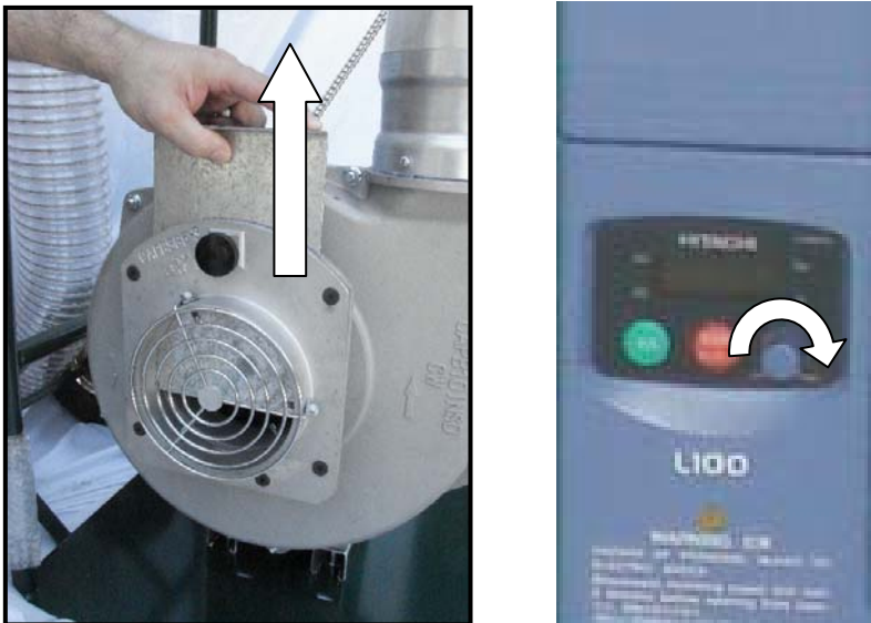
Figure 14 – Obtaining System Test Pressure
