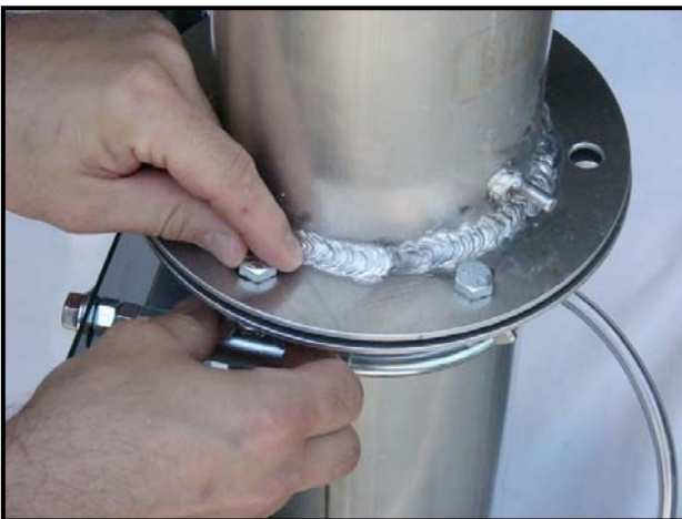
Figure 3 – Bolting Flange (hand tighten snugly)
